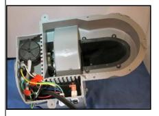
120V power is passed from the control – to the yellow wire – and to the blower motor. This yellow wire is the only source of AC power for the blower motor.
