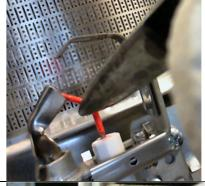
4. When completed, the igniter rod should be positioned in the middle of the notch (saddle) of the pilot hood; and ½ inch from the hood. (Use a drill bit or Allen wrench as a gauge.)
