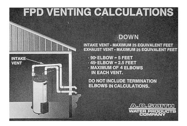
Down Venting Calculations: FPD Intake and exhaust elbows must be on same surface of the house. Excluding the vent terminations, a maximum of 25 equivalent feet may be used in the intake vent system and a maximum of 25 equivalent feet may be used in the exhaust vent. However, excluding the termination elbow, you can have no more than four elbows in each vent.
