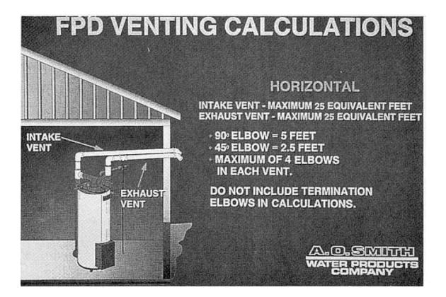
Horizontal Venting Calculations: FPD The FPD Sealed Shot features a two pipe system with a fresh air intake vent and an exhaust vent. Intake and exhaust elbows must be on same surface of the house. A maximum of 25 equivalent feet may be used in the intake vent system and a maximum of 25 equivalent feet may also be used in the exhaust vent. However, excluding the termination elbow, you can have no more than four elbows in each vent.
