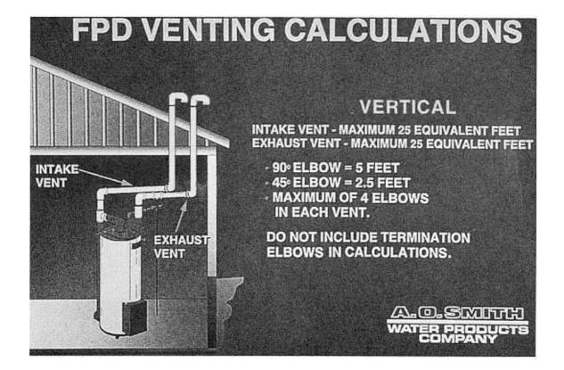
Vertical Venting Calculations: FPD This unit is approved for venting through the roof with only the terminations supplied with the unit. Intake and exhaust elbows must be on same surface of the house. Excluding the vent terminations, a maximum of 25 equivalent feet may be used in the intake vent system and a maximum of 25 equivalent feet may be used in the exhaust vent. However, excluding the termination elbow, you can have no more than four elbows in each vent.
