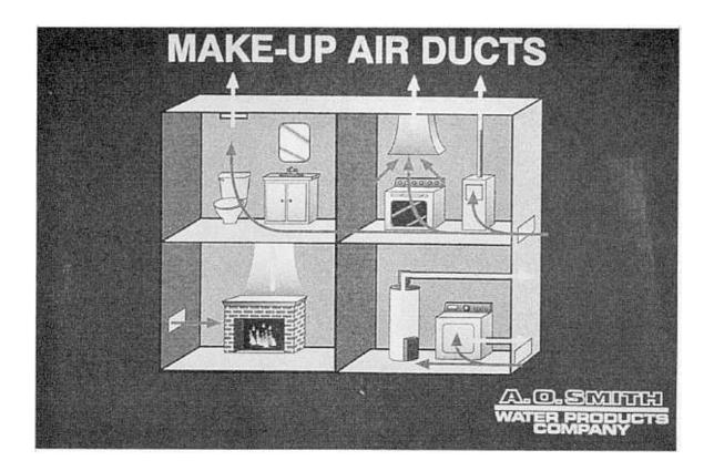
Make-up Draft To alleviate a negative pressure condition, install makeup air ducts (per makeup air specifications listed in the National Fuel Gas Code) of sufficient capacity to allow all appliances requiring makeup air to operate properly.
