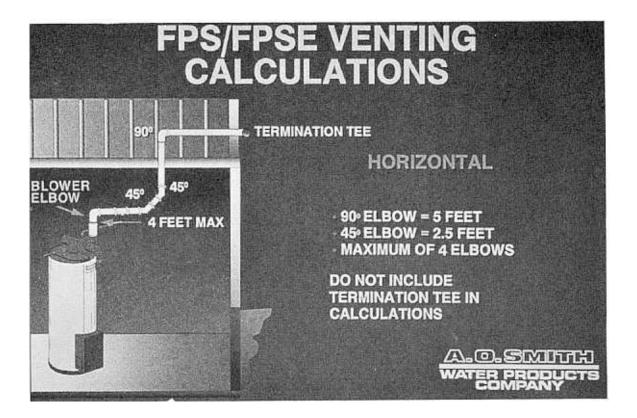
Horizontal Venting Calculations: FPS FPSE As you can see, the FPS & FPSE40 - 50 models allow for increased venting flexibility. They can be vented horizontally up to a maximum of 45 equivalent feet from the heater. Do not include termination tee in calculations.
