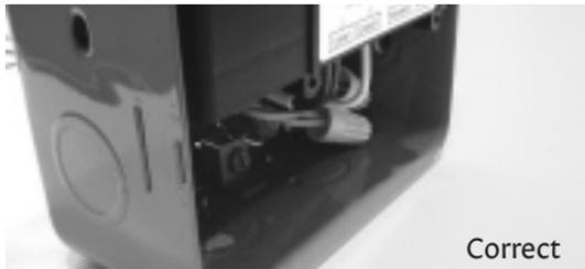
9. If using a smaller sized enclosure, it will be necessary to snap the Plexiglass® insulator along the scratch line for proper fit. With safety glasses on, simply place the line along a table edge, hold firmly in place and apply pressure to the overhanging section of Plexiglass® until it snaps apart (see images below).
