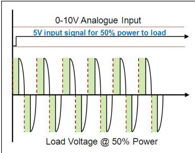
Figure 3; Simplified Phase-Angle Waveform at 50% Power
