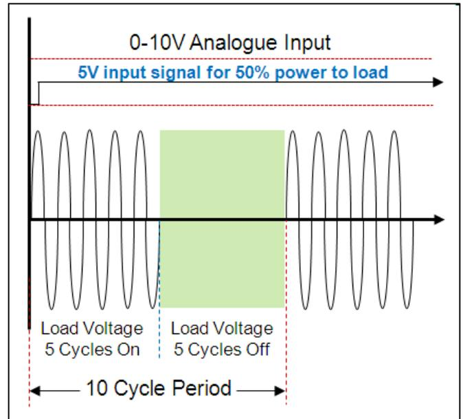
Figure 4; Simplified Burst-Fire Waveform at 50% Power
