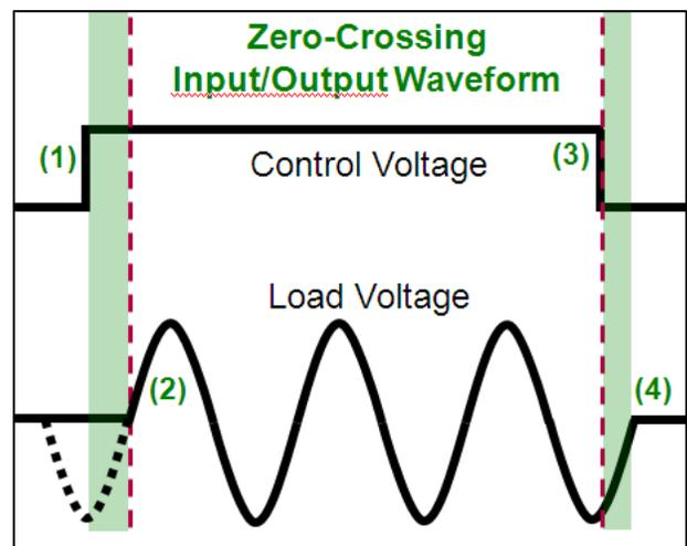
Figure 1; Simplified Zero-Cross Waveform
