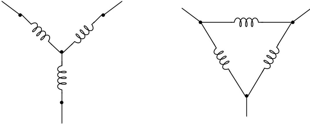
In which circuit (Y or Delta) are the phase and line currents equal? In which circuit (Y or Delta) are the phase and line voltages equal? Explain both answers, in terms that anyone with a basic knowledge of electricity could understand.
