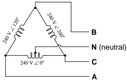
Identify the different voltages obtained from this coil configuration, and which connection points each voltage is measured between.
