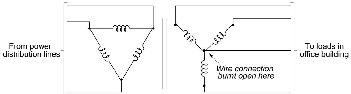
What is strange, though, is that the overheated wire is the *neutral* conductor, not any one of the "line" conductors. Based on this observation, what do you think caused the failure?
