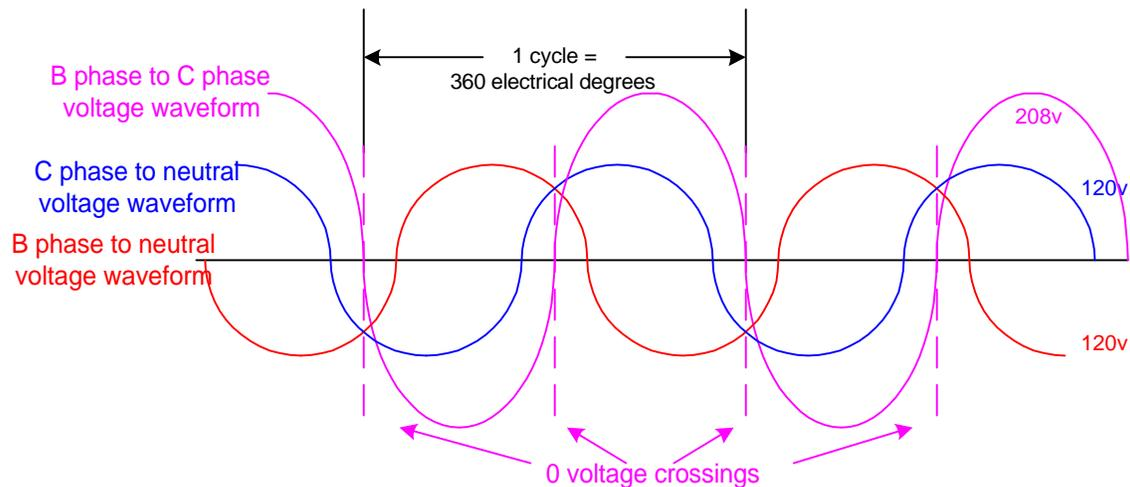
The B phase to C phase waveform shown in purple is a single phase, 208 volt relationship that exists in the output from the transformer on the previous page. The waveform produced by the relationship between A phase and C phase, is very similar to this one, except that it occurs 120 electrical degrees away. Likewise, the waveform for A phase and B phase makes up the third “leg” of this three phase, 208 volt transformer output.
