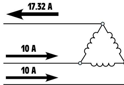
**Figure 12-15** Division of currents in a delta connection.
