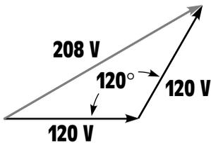
**Figure 12-11** Adding voltage vectors of two-phase voltage values.
