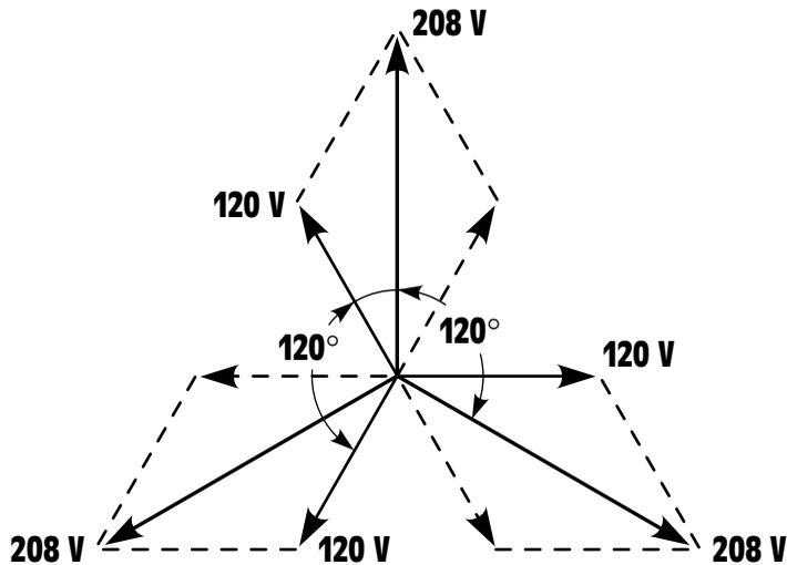
Figure 12-12 The parallelogram method of adding three-phase vectors.
