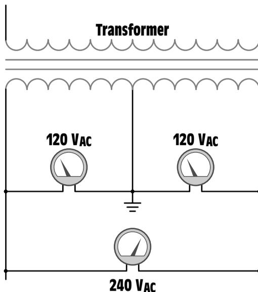
**Figure 12-8** Single-phase transformer with grounded center tap.
