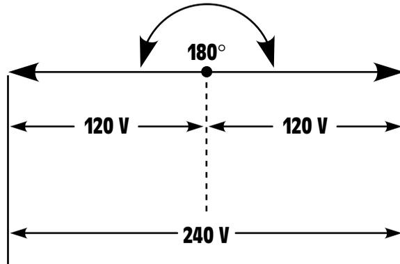
**Figure 12-9** The voltages of a single-phase system are  $180^\circ$  out of phase with each other.
