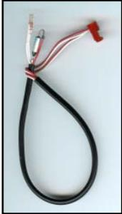
The high limit switch opens after flame is established. That means the water in the tank got over 200<sup>0</sup>F.
