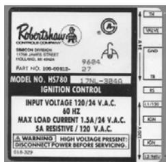
One of the major differences with the hot surface ignition is the Robert Shaw HS 780 Electronic Ignition Module. The module comes in a 'one try' and a 'three try' model. The HS780 ignition control is a direct main burner ignition system that provides the timing sequence, along with the ability to sense main burner flame.
