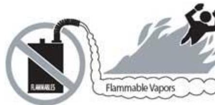
Turn off water heater when working with fuel, paint, glue, and flammables
