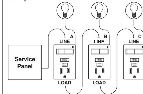
Placing the GFCI in position A will also provide protection to "load side" receptacles B and C. On the other hand, placing the GFCI in position C will not provide protection to receptacles A or B. Remember that receptacles A, B, and C can be in different rooms.
