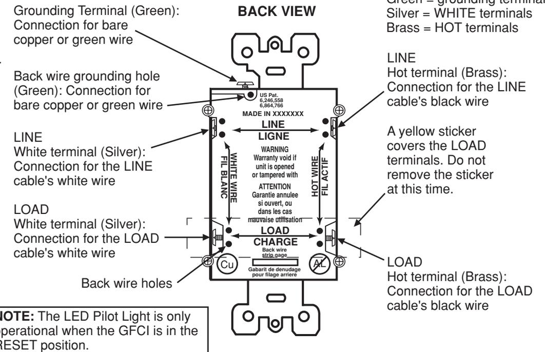
**NOTE:** The LED Pilot Light is only operational when the GFCI is in the RESET position.
