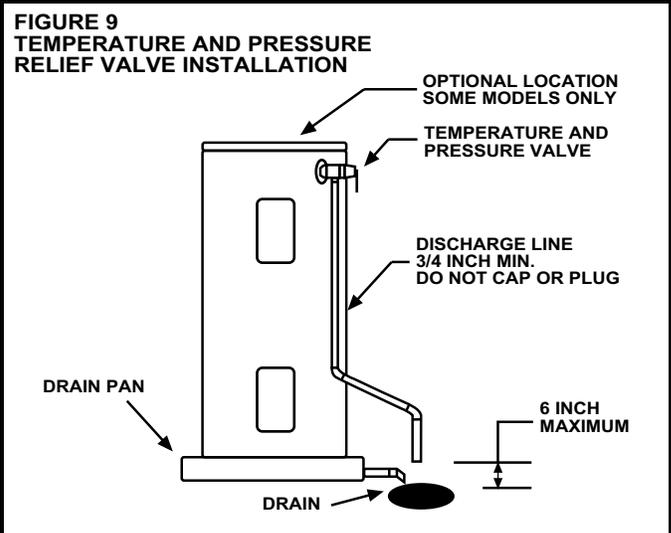
For protection against excessive pressures and temperatures, a temperature and pressure relief valve must be installed in the opening marked "T & P RELIEF VALVE" (See Figure 9).
