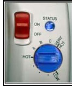
Notice the BLUE temperature adjustment knob. That is how you identify the proper gas control for this product.
