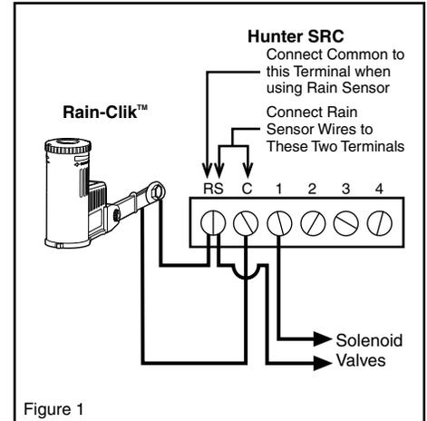
**Wiring to the Hunter ICC, Pro-C, or EC Controllers**
