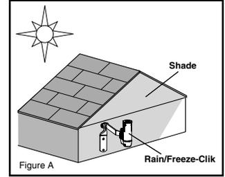
Once the Rain-Clik is mounted, run the wire to the controller, and fasten it every few feet with wire clips or staples for best results. Be careful not to cut through the wire insulation with fastening hardware or chaff the insulation when routing wire through or around metal materials (i.e. gutter, siding, etc.). If an extension to the wire provided is needed, use the following table to determine the minimum wire gauge needed:
