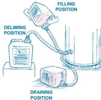
**Part No. 4813-3** - Residential Use - Complete kit includes vented plastic jug, tubing, clamps, fittings, instructions and 3 gallons of UN•LIME Delimer for small and medium residential water heaters.
