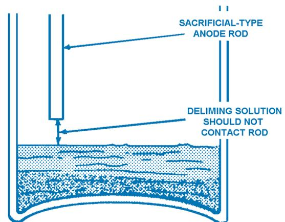
**FIGURE 3 - DELIMER SHOULD NOT CONTACT SACRIFICIAL-TYPE ANODE**
