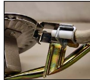
Figure 6 – Ignitor Assembly
