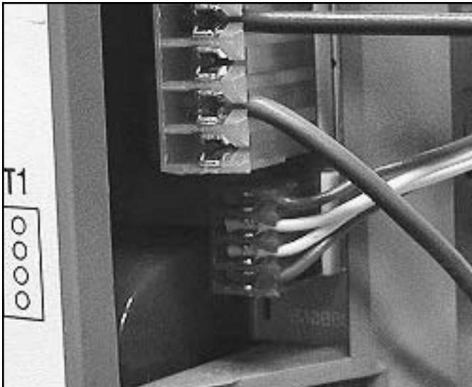
1. Remove the red molex plug. Measure OHMS resistance between the two white wires on the plug.
