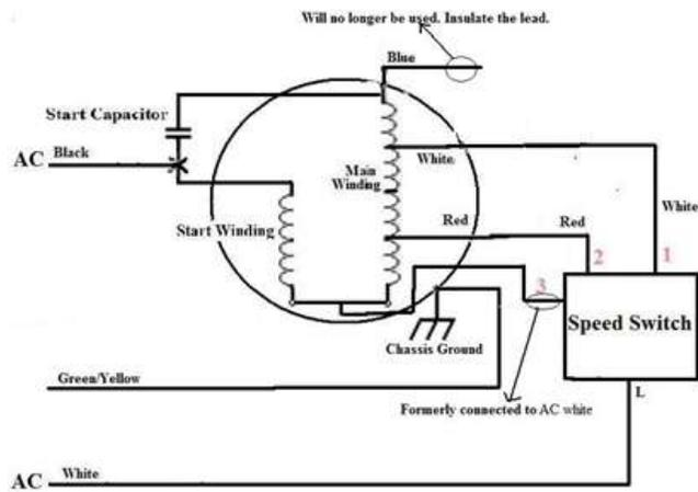
Below are the wiring modifications for 2-speed and single speed single phase capacitor-start electric motors.
