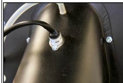
120V power is passed from the control to the blower motor on the yellow wire on the gas control.
