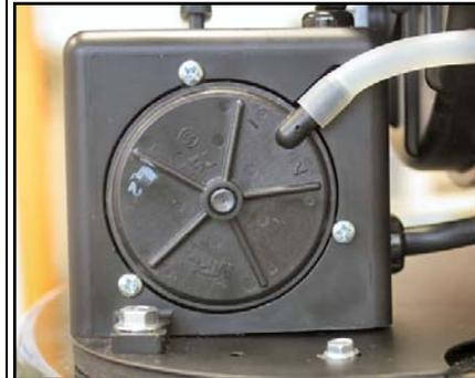
A signal is passed thru the pressure switch to the control valve.
