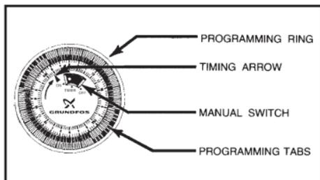
1. Set the timer switch to the actual time by turning the programming ring in the direction of the arrow until the timing arrow points to the actual time on the ring.
