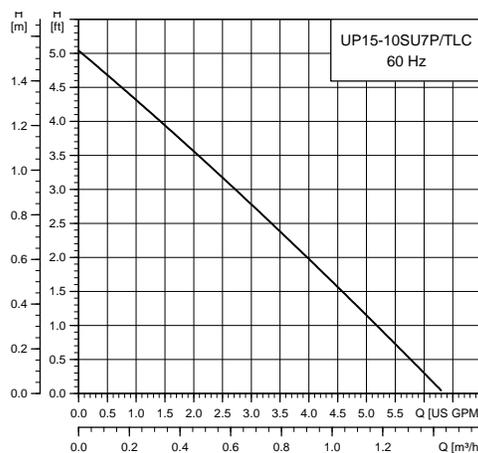
Fig. 8 Performance curve for the Comfort System
