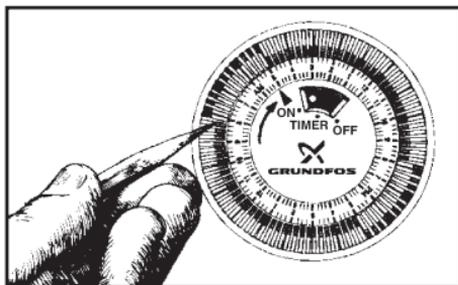
5. For continuous operation, set the manual switch to the “ON” position. To switch the circulator off, set the manual switch to the “OFF” position. The “ON”/“OFF” modes may be used without affecting the function of either the programming ring or the timer switch.
