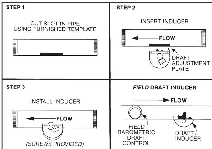
**FIGURE 25: Inducer mounted vertically**
