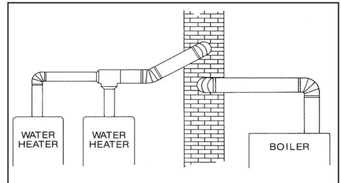
**Figure 24: Determining the use of a 5” common gas vent**
