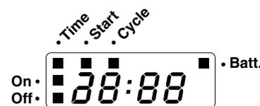
If the battery voltage falls below a certain level the **Batt.** indicator appears. It is possible to initiate watering manually even if the battery capacity is too low (valve no longer opens), but programmed watering times, however, are not initiated.
