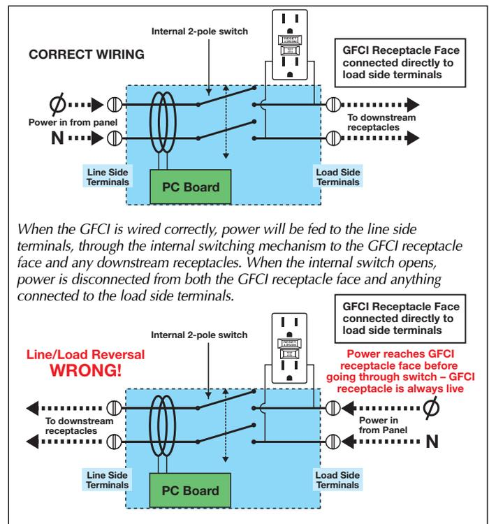
When the GFCI is wired correctly, power will be fed to the line side terminals, through the internal switching mechanism to the GFCI receptacle face and any downstream receptacles. When the internal switch opens, power is disconnected from both the GFCI receptacle face and anything connected to the load side terminals.
