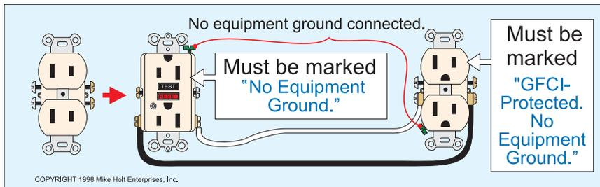
For increased electrical safety, Leviton strongly recommends installing a GFCI in every non-grounding circuit. A ground wire provides protection by offering a parallel path back to ground for any fault
