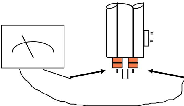
If the reading is less than 20 ohms on the "Rx 1" scale or the "Rx 10" scale the element is good, if it is much greater e.g.... 10,000 ohms or if you get a reading on the "Rx 1K" scale then you must replace the element (contact Eemax).
