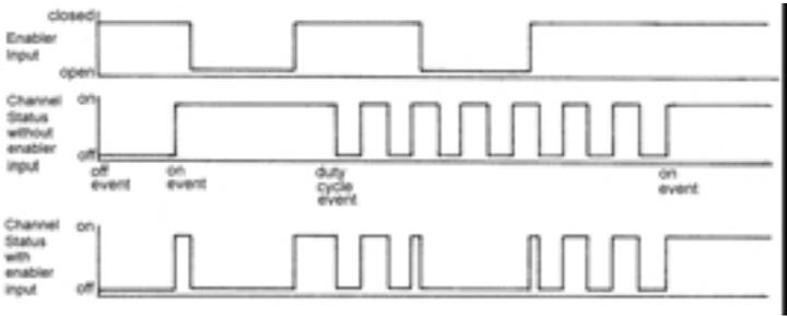
**Example No. 4**                      Operation of On\d (On with off delay) override input
