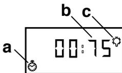
The countdown timer can be set to turn the plugged in light(s) on or off after 75, 60, 45, 30 or 15 minutes. That lets you, for example, set the timer to turn the plugged in light(s) off an hour after you have left the room. The flashing alarm clock symbol indicates the DT11 is in countdown timer mode.
