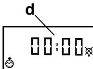
When the countdown reaches 00:00 the connected light(s) are switched and the clock display remains 00:00 (d).
