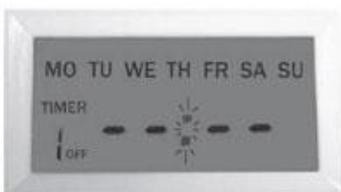
2. Using the **h+** and **m+** keys, enter the desired OFF time. By default, all days are indicated. When complete, press the **Timer** key once.
