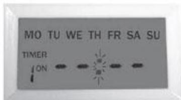
1. Using the **h+** and **m+** keys, enter the desired ON time. By default, all days are indicated, thus all 7 days will be programmed. When complete, press the **Timer** key once.
