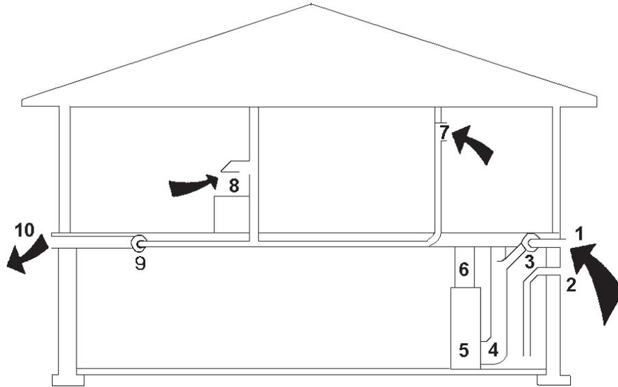
*A neutral pressure mechanical ventilation system for a tight house uses several fans and ducts as in this example: 1) a powered intake for outdoor air; 2) a passive intake for outdoor air; 3) a fan for the intake; 4) the cold air plenum for the furnace; 5) the furnace blower; 6) the warm air plenum for the furnace; 7) the bathroom exhaust fan; 8) a kitchen exhaust register; 9) an exhaust fan; and 10) an exhaust damper. The power intake and exhaust are wired to operate together*
