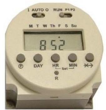
Clear timer: Press Reset with paper clip and hold for few seconds. Repeat. Minimum time setting 1 minute. Lithium battery provides 5 year backup.
