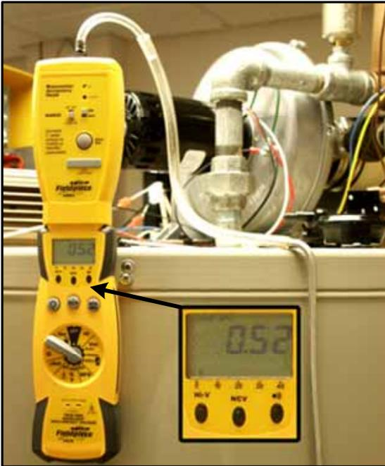
**Blocked Exhaust Switch Pressure Test
