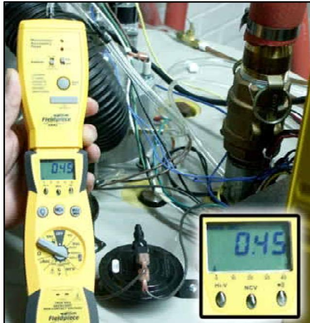
**Blocked Exhaust Switch Pressure Test
