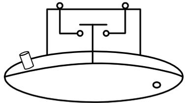
Normally closed contacts, open on a fall in pressure.
