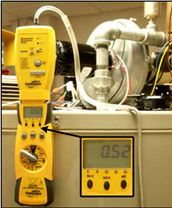
Blocked Exhaust Switch Pressure Test Cyclone - BTH 300/400 Models
