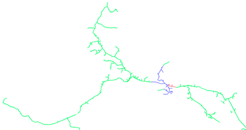
Figure 19. Real distribution feeder with regions of compliance (green), undervoltage (red) and overvoltage (blue) highlighted for the maximum loading case on the network with the optimal tap settings applied.
