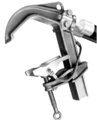
C600-0337 Aluminum Body, Smooth Jaws, Bronze Eyescrew, Pressure Type
