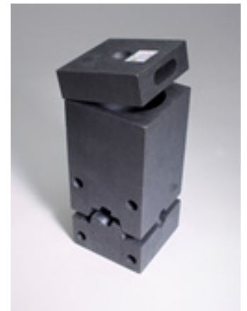
Figure 2.2-7 A graphite mold for exothermic welding. The reaction is initiated by igniting powder at the opening on the top of the mold.
