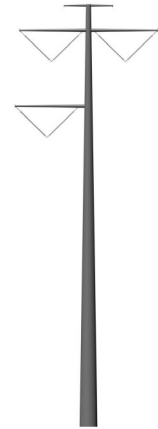
500-kV single-circuit TSP
