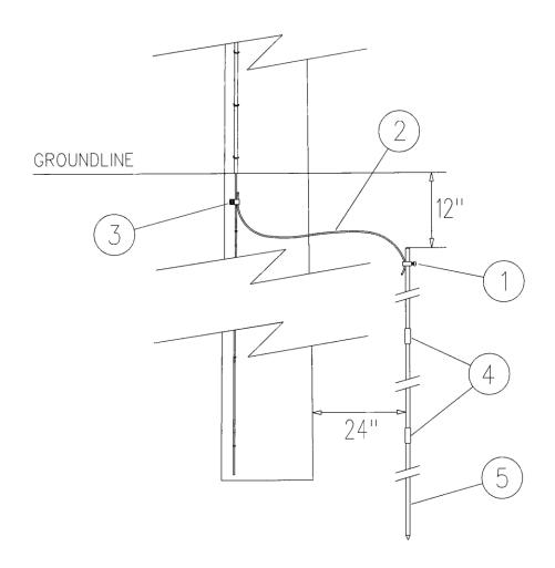
NOTE: EXISTING GROUND-WIRE SHOULD BE CUT AND ATTACHED DIRECTLY TO THE GROUND ROD IF POSSIBLE. IF THIS CANNOT BE DONE, BUILD AS SHOWN.
