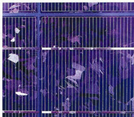
Photovoltaic cells, which generate electricity directly from sunlight, are made of polycrystalline silicon. The array of cells above is installed at Montgomery College in Germantown, Maryland. A detail, below, shows the grain structure of the silicon material and the grid of metallic conductors laid down over it to collect current.
