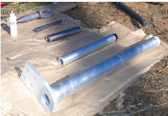
Figure 5-11 Dead-end fittings hardware used for ACCC conductor
