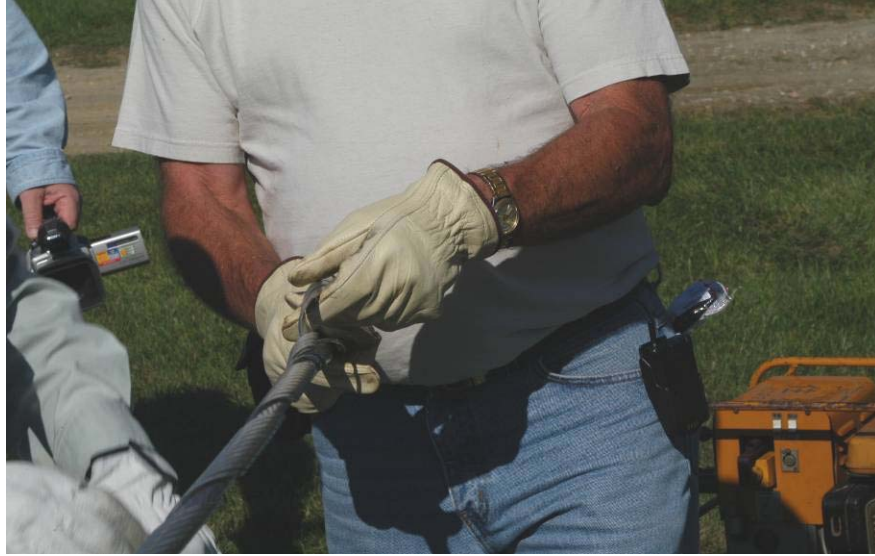
Figure 5-4 Removal of gap conductor strands at the termination at the EPRI Lenox Lab
