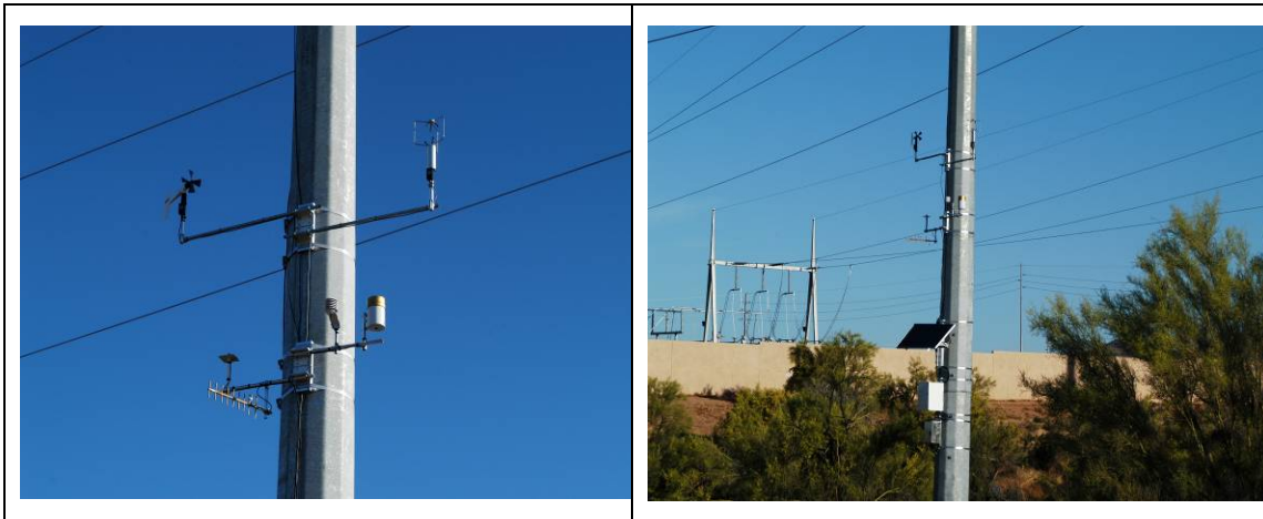
Figure 7-2 Ambient condition measurements from a set of instruments: anemometer, rain gauge etc. powered through a solar panel
