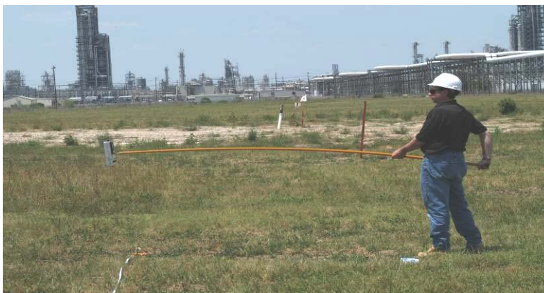
Figure 7-5 EMF measurement process under a transmission line
