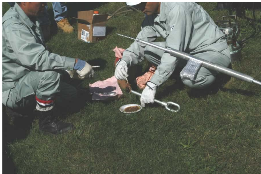
Figure 5-5 Application of high-temperature grease on core-grip portion
