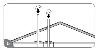
Install adequate flashing where the vent pipe passes through the roof.
