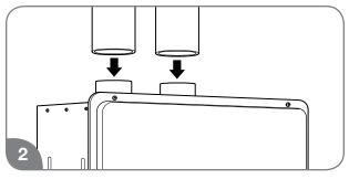
Complete the vent pipe installation to the water heater's vent connector fittings. Use cleanerprimer and PVC cement where the vent pipes join the water heater.
