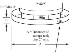
This line should be at least 3/4" ID and pitched for proper drainage to an open drain.
