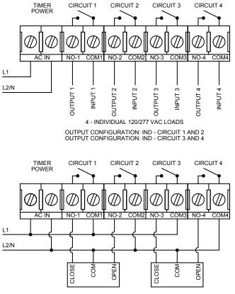
TIMER CONFIGURATION FOR TWO CONTACTOR CONTROLS OUTPUT CONFIGURATION: PUL - CIRCUIT 1 AND 2 OUTPUT CONFIGURATION: PUL - CIRCUIT 3 AND 4
