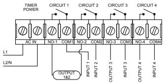
TIMER CONFIGURATION FOR COMBINATION MODE OUTPUT CONFIGURATION: SIM - CIRCUIT 1 AND 2 (208/240 VAC LOAD) OUTPUT CONFIGURATION: IND - CIRCUIT 3 AND 4 (120/277 VAC LOAD)
