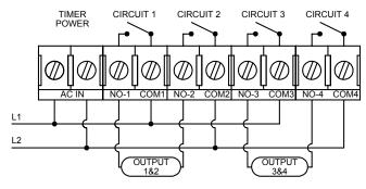
TIMER CONFIGURATION FOR TWO 208/240 VAC DSPT OUTPUT CONFIGURATION: SIM - CIRCUIT 1 AND 2 OUTPUT CONFIGURATION: SIM - CIRCUIT 3 AND 4
