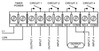
TIMER CONFIGURATION FOR COMBINATION MODE OUTPUT CONFIGURATION: IND - CIRCUIT 1 AND 2 (120/277 VAC LOAD) OUTPUT CONFIGURATION: SIM - CIRCUIT 3 AND 4 (208/240 VAC LOAD)
