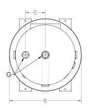
\*Note: These connections are not for piping connections. They are the anode locations and also serve as the required ASME 2" inspection openings.
