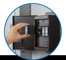
Step 1 Turn off power and remove affected module
