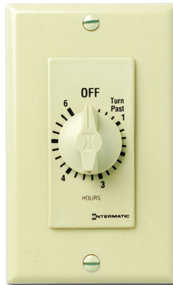
Spring Wound Countdown Timer, Decorator Style, 125-277 VAC, 50/60 Hz, SPST, 6 Hour Max, Without Hold, Ivory
