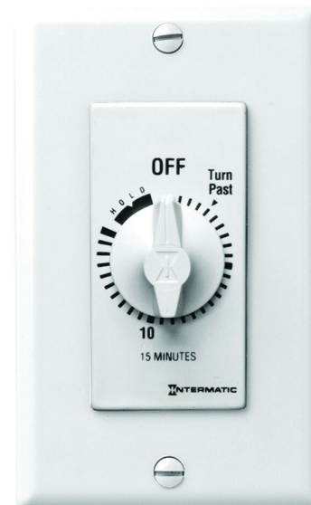
Spring Wound Countdown Timer, Decorator Style, 125-277 VAC, 50/60 Hz SPST, 15 Minute Max, With Hold, White
