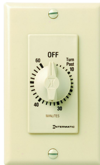
Spring Wound Countdown Timer, Decorator Style, 125-277 VAC, 50/60 Hz SPST, 60 Minute Max, Without Hold, Ivory
