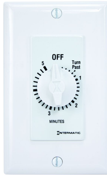
Spring Wound Countdown Timer, Decorator Style, 125-277 VAC, 50/60 Hz, SPST, 5 Minute Max, Without Hold, White
