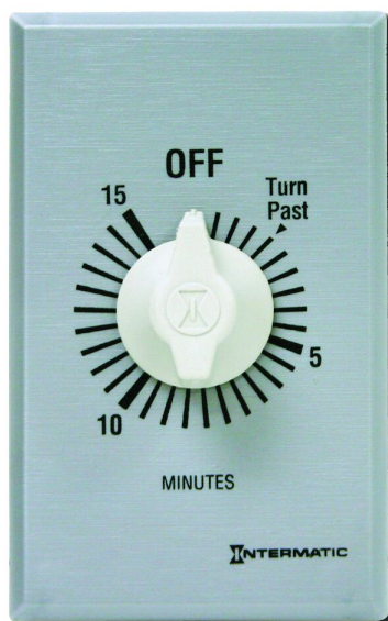
Spring Wound Countdown Timer, Commercial, 125-277 VAC, 50/60 Hz DPST, 15 Minute Max, Without Hold, Silver
