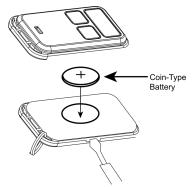
Figure 5 Removing transmitter cover
