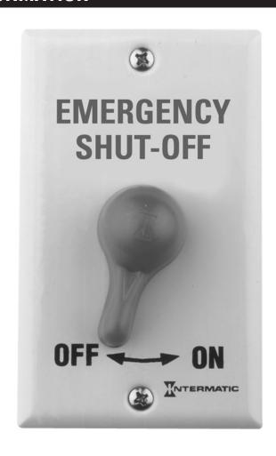
This Switch is designed to be installed in a standard flush or over the surface indoor/outdoor single gang 1½ inch or deeper junction box. The method of installation, as well as the location, must conform to the National and Local Electrical and Building Codes. If not sure, please consult your local inspection authorities prior to installation.
