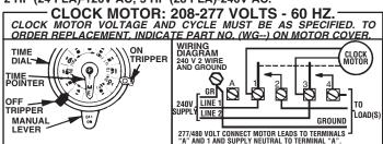
WIRING INSTRUCTIONS: To wire switch follow diagram above. Use solid or stranded COPPER only wire with insulation to suit installation. See gauge selection table for normal service applications. To make power connections remove 1/2 inch of insulation from wire ends. Insert bare ends of wire under the pressure plate of terminals. Use 3/16 or larger screwdriver to tighten terminal screws firmly. (25 lb-in minimum).
