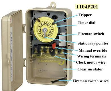
Heater protection circuit: 10A 240V max. WG1573 clock motor/ 156T1978A Tripper / 9-3/8" H x 5-1/2" W x 3-5/8" D/ ½" and ¾" KO on back and side
