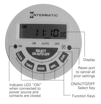
**To Override Automatic Operation Permanently:** Press SELECT key to move indicator bar to the desired ON or OFF position. **Note: Timer will not resume** automatic
